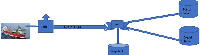
Typically, slop is not sold. It is tested and a blending plan put in place (in collaboration with the NPA) to restore its quality and sold as normal products. In fact, users of petroleum tank farm facilities hardly hear of slop and the management of it.
